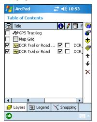
can reorder the layers, turn layers on and off, and change the color of layers, among other things. The column of checkboxes under the eye icon control layer visibility. Tap a layer's name to select it, and tap the up and down arrows to move it up and down (the layers draw from the bottom up, so the higher-up layers will draw on top of the lowerdown layers), or tap the Properties button (on the right, just
