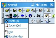
from the top. The first dropdown toolset has the Zoom In, Zoom Out, Pan, and Rotate Map tools. Tap the dropdown arrow and tap a tool to select it; it will appear pressed-in. Now tap or tap-and-drag on the map display to use the tool. The second and third dropdown toolsets on the second toolbar contain additional zooming buttons (these do not need to be selected and then used on the map display like the tools in the first dropdown toolset – they function
